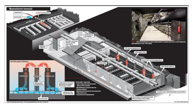
The cooling is organized with cold and hot aisles, which prevents the cold air flow led to the servers from mixing with the heat produced by the servers. In addition, server racks are isolated from each other and placed in solid rows with no empty spaces between the racks, which further decreases the need of cold air flow. The cooling is optimized using big data it collects from the data center.
